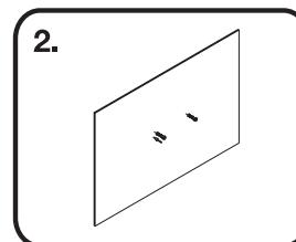
Drill two holes then insert the expansion bolts to the holes.
